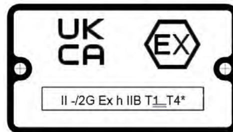
Figure 11: Typical UKCA Ex nameplate
