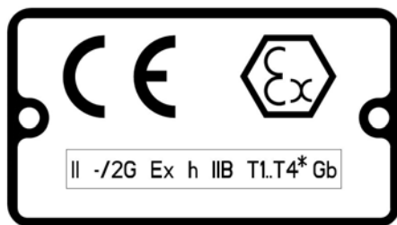
Figure 10: Typical Ex nameplate
