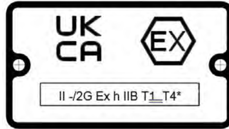
Figure 2: Typical UKCA Ex nameplate
