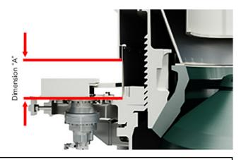
Caution: A is given for a good wear. Meaning similar mantle and concave wear, without distorted wear profile = correct application according to cavity selected.
