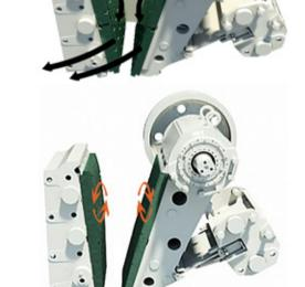
Note: Cupping may occur in the joint of movable jaws if the movable jaw is rotated when it is installed in the lower position. This may decrease the crusher's capacity and increase wearing on the fixed side.
