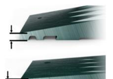
Jaws with locking wedges in the back can wear to a thickness of 60-65 mm until they must be changed.
