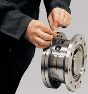
1 Remove old shear tube.
