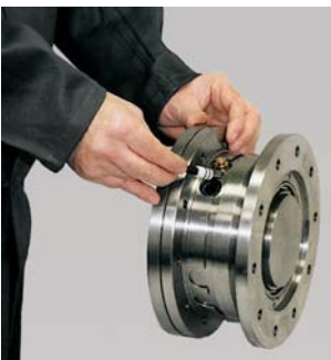
3 Remove sealing plug from injector connection.
