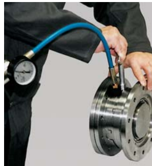
5 Pump up until required pressure is reached, re-tighten shear tube firmly.
