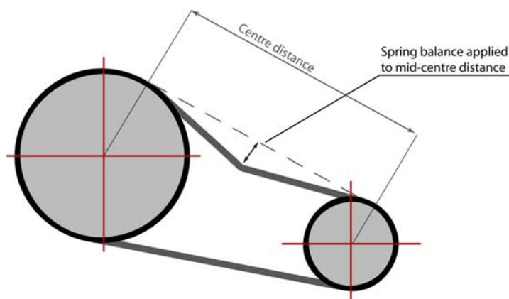
Figure 3: Belt tensioning diagram
