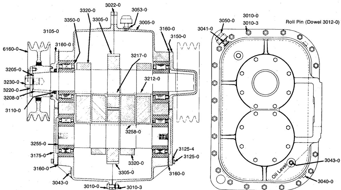
Figure 4.1 Typical Cross Section through Low-Head Mechanism.
