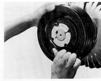
*Removing a Taper Lock® bush*
