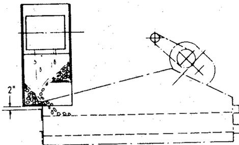
For de-watering and de-sliming, with baffles in feed chute to reduce feed velocity.
