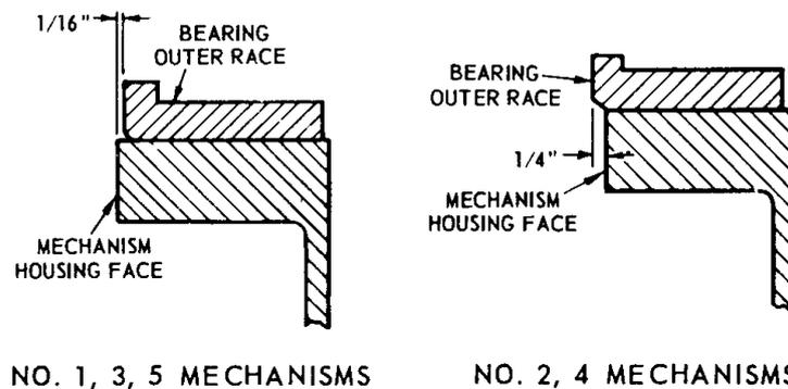
Figure 4.9 Position of bearing outer race in relation to mechanism housing face before assembling bearing caps.
