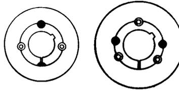
2. Insert screws in jacking off holes after oiling thread and point of grub screws or thread and under head of cap screws.
