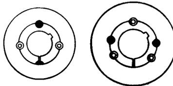
3. Clean shaft and fit hub to shaft as one unit and locate in position desired, remembering that bush will nip the shaft first and then hub will be slightly drawn on to the bush.
