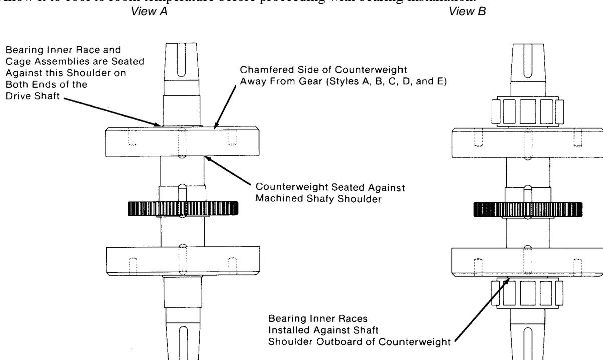
Figure 4.6 Installation of second counterweight and bearing inner races with roller cage assemblies on drive shaft.
