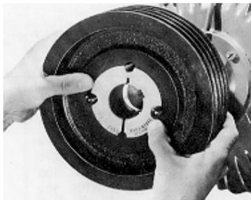
*Insert screws and locate on Shaft*
