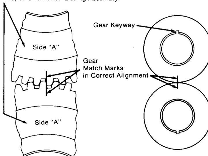
*Figure 4.10 Match mark alignment of properly assembled gears.*
