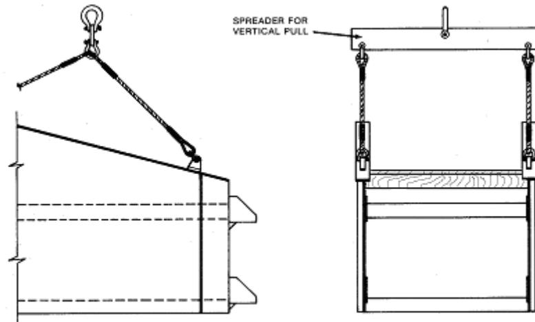
*Figure 1.1 Use of spreaders when lifting the screen*
