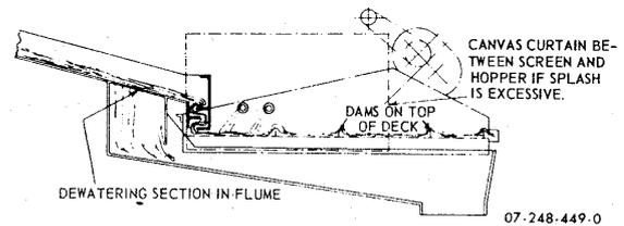
For de-watering and de-sliming, with baffles in feed chute to reduce feed velocity.
