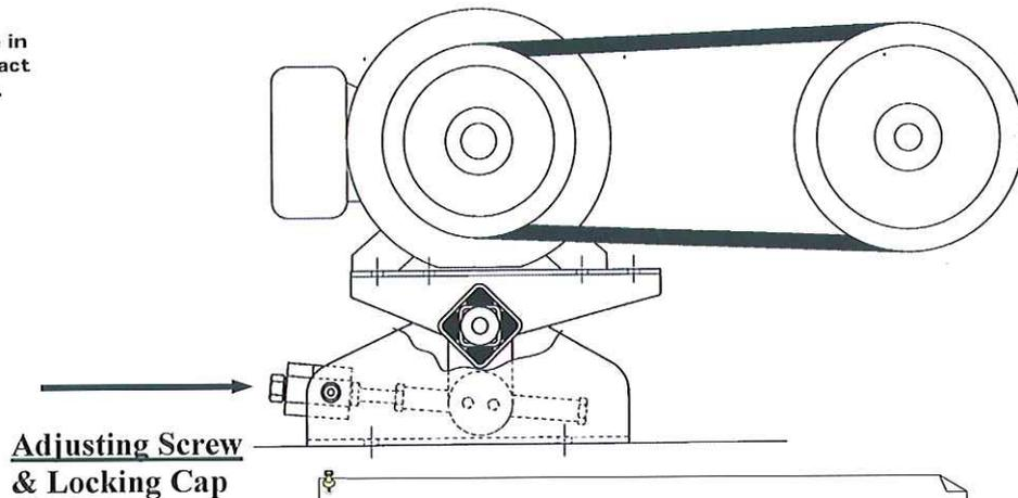
Leverlink Motor Bases have been developed to simplify the changing and retensioning of Vee Belts. We recommend the use of a *Ratchet*, which will allow the Vee Belts to be adjusted or changed quickly and efficiently.
