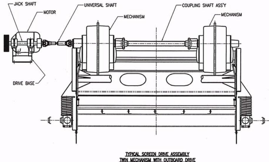
*Figure 2.4 - Cardan Shaft /Jack Shaft Arrangement*
