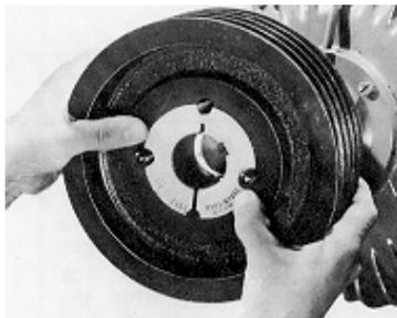
Insert screws and locate on Shaft
