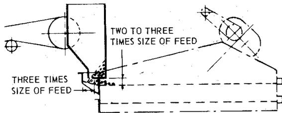
For small material (2.5" max.), using feed box.
