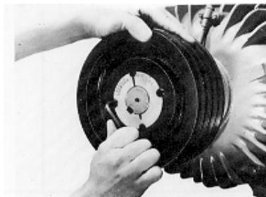
Tighten screws alternately
